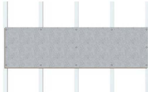
④ Screw pattern for panel widths of 600 mm and 850 mm
